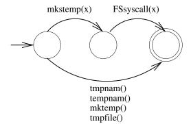
Figure 3. An FSA to detect insecure uses of temporary files.
