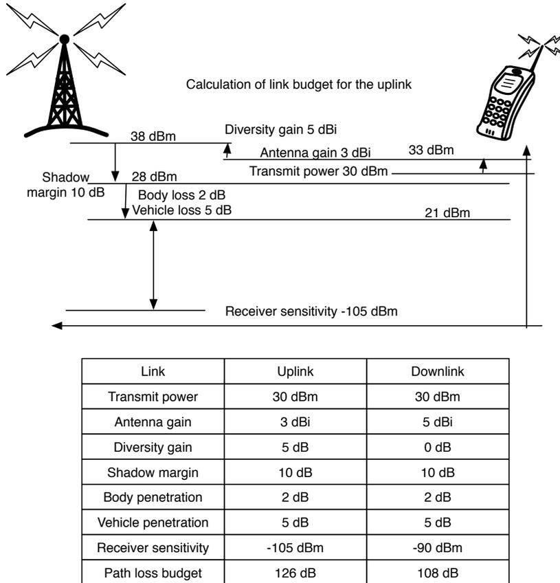
**Figure 13.10** Illustration of link power budget.
