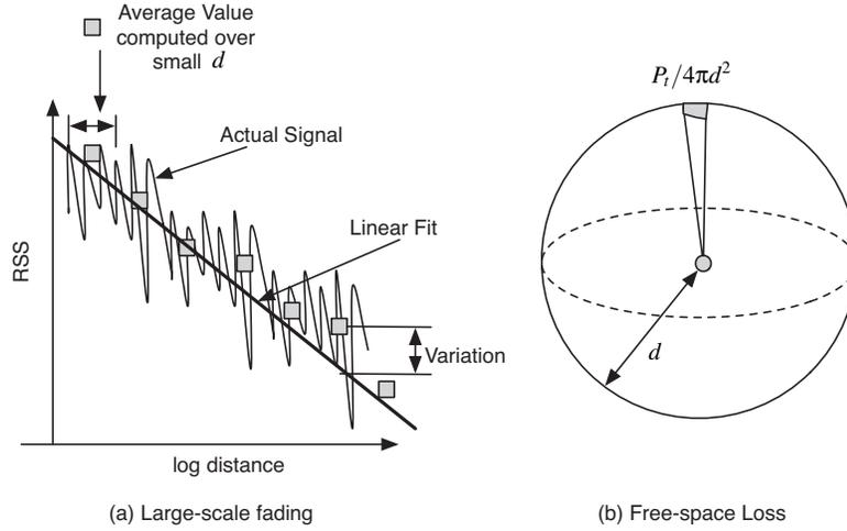
**Figure 13.6** Large-scale fading and free-space loss.
