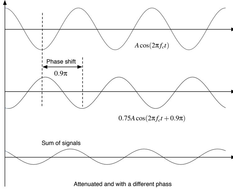
**Figure 13.7** Illustration of fading.
