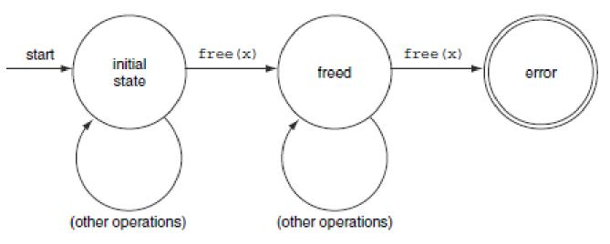
Model checking will look for a variable wrt which system will reach state error
