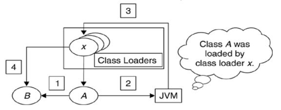
Prevents less trusted replacing more trusted ..
