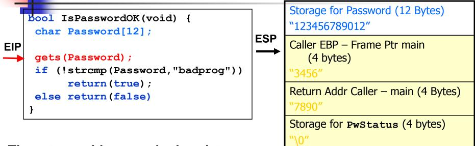
The return address and other data on the stack is over written because the memory space allocated for the password can only hold a maximum 11 character plus the NULL terminator.
