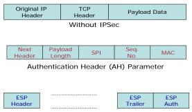
Encapsulating Security Payload (ESP) components
